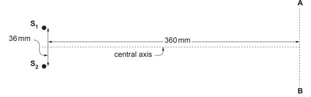
Use the equation for double slit interference to determine the approximate spacing between points of maximum microwave intensity. [2]
